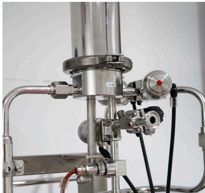
Conventional construction of a filter base with process valves welded on
