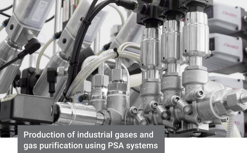
Valve solutions for pressure swing adsorption systems
