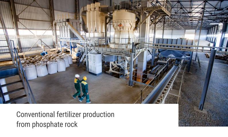
The production of phosphate fertilizers goes hand in hand with the production of mineral acids. Most important are phosphoric acid (as an intermediate or major product), sulphuric acid (as a major reagent), and nitric acid (as a reagent or additive).
